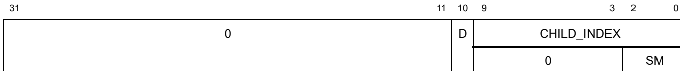
Figure 8.8 Source Configuration Register Bit Assignments
