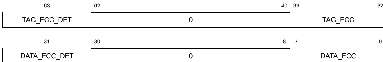
Figure 5.31 Global L2 ECC Register Bit Assignments
