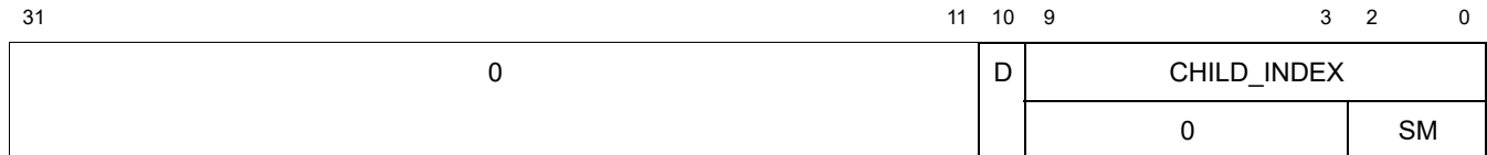
Figure 8.8 Source Configuration Register Bit Assignments
